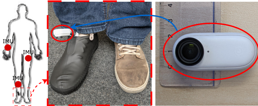
Fig. 1. The foot-mounted camera captures localized ground context for terrain-aware activity recognition while naturally reducing the capture of surrounding people and scenes.
